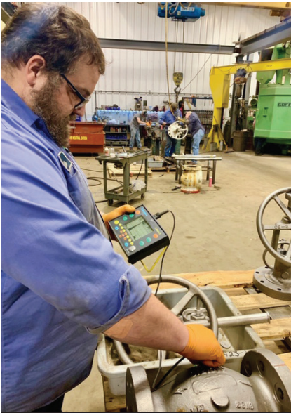
□ Wall thickness checks on valve bodies can help to ensure they meet customer specifications.
