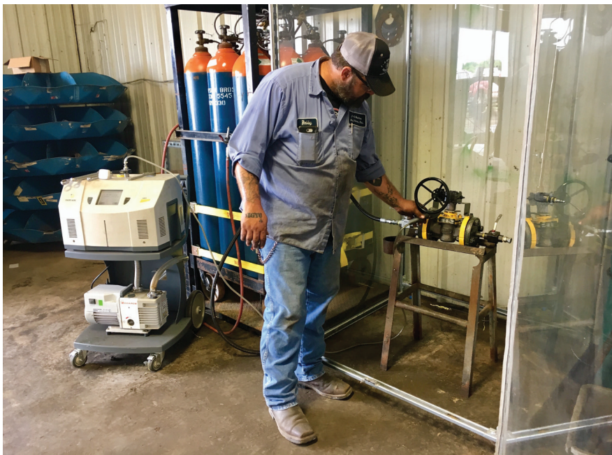
□ A mass spectrometer helps to meet stringent, helium valve testing requirements.
