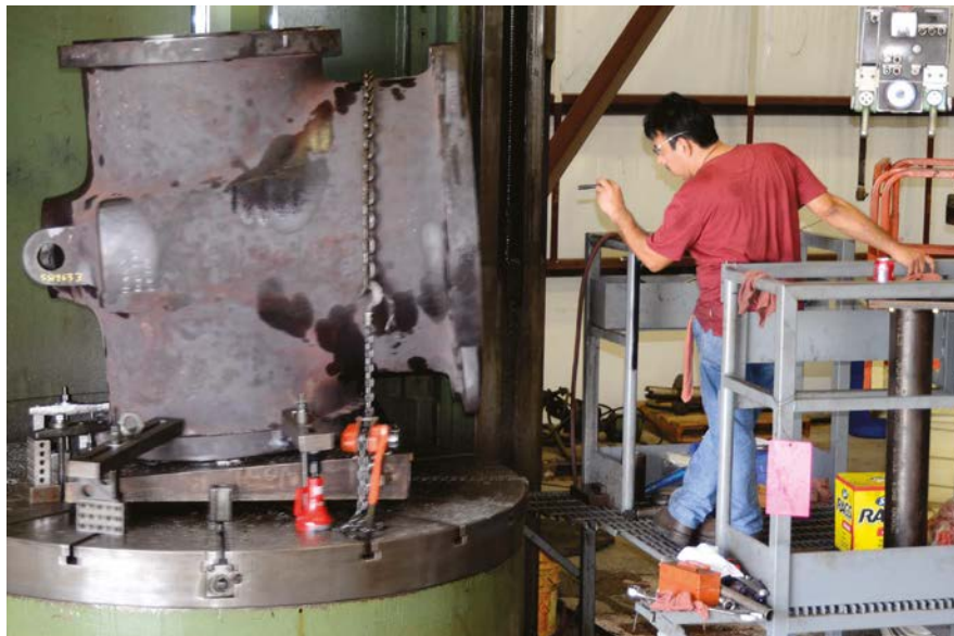
□ The seats of a 30-inch gate valve are machined before weld overlay for a hardfacing modification.
