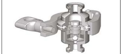
Figure 3. Cutaway showing clean steam trap construction
