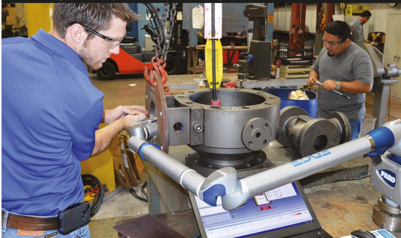
□ A coordinate measuring machine is used to verify that modified valve components meet OEM drawing dimensions.
