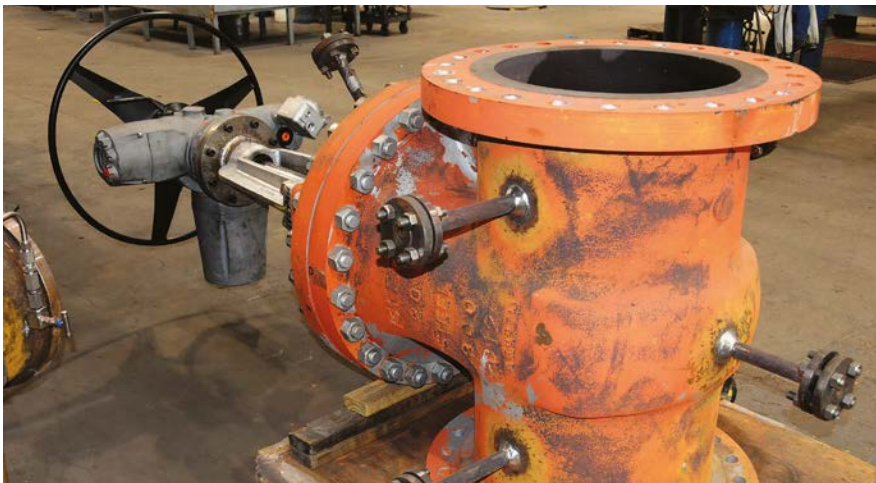
□ A gate valve has been modified by welding multiple drains on the body. The discoloration is a sign that the body has been stress-relieved after welding
