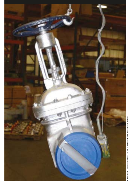
Figure 3. How NOT to lift a gate valve
