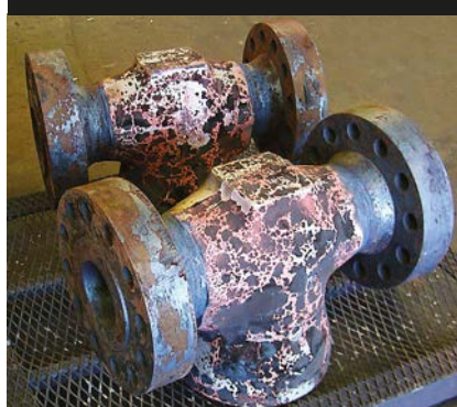
□ These valve bodies have been removed from the furnace following a post-weld heat treatment.
