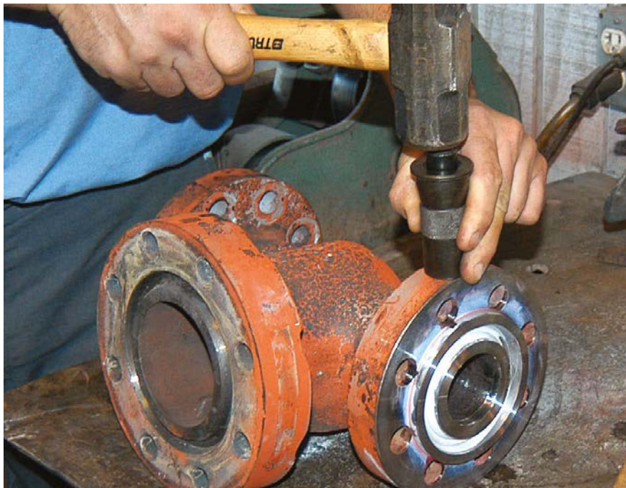
□ A hardness test is performed on a valve body following a heat-treating operation.
