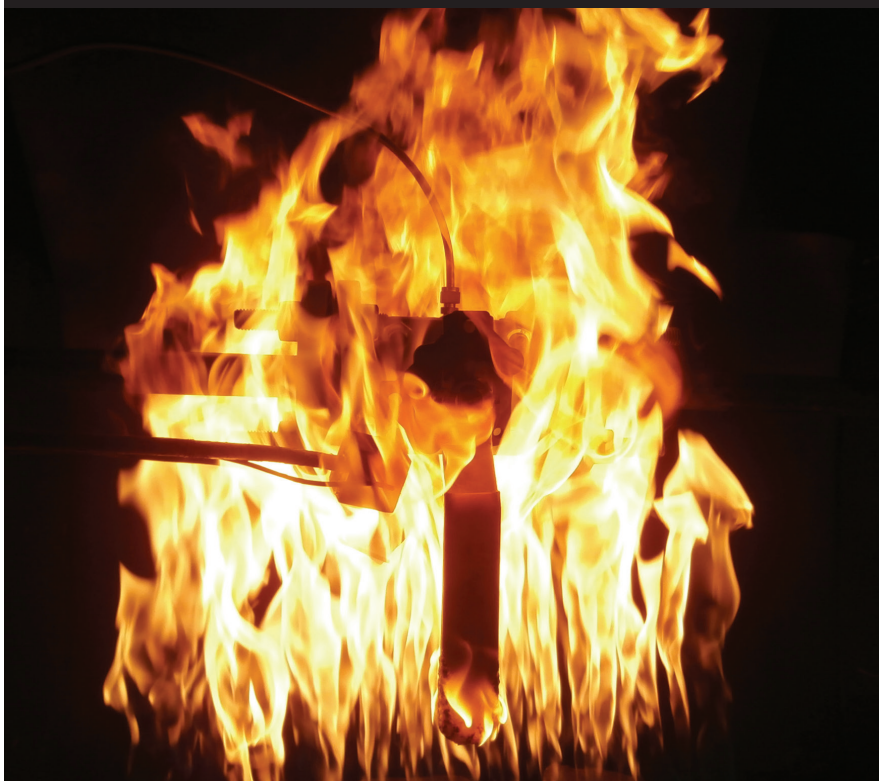
□ Ball valve during API 607 test
