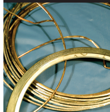
□ A delaminated spiral-wound gasket is shown next to the pristine replacement gasket. Delamination can cause catastrophic leaks and damage downstream piping components.
