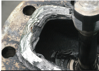
□ This is an example of a failure of a graphite-laminated soft steel gasket on a Class 150 gate valve. The failure created a catastrophic leak.
