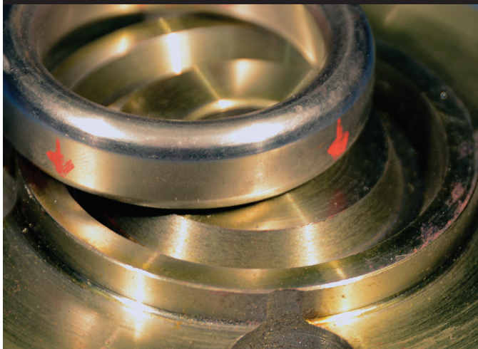
□ RTJ gaskets require carefully machined smooth grooves in order for the metal gasket to seal properly. The RTJ gasket must also be softer than the groove material so it can slightly deform into the groove area.
