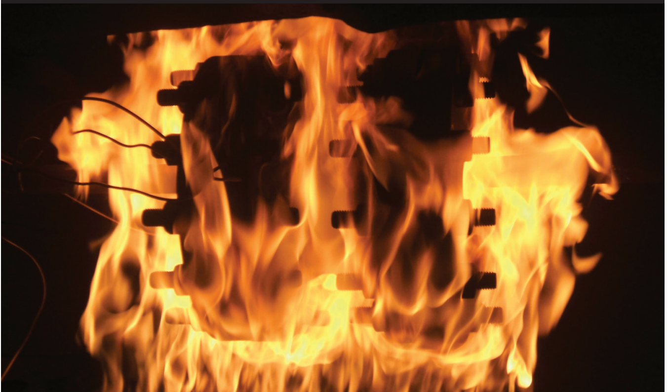
□ Figure 4. Exxon-modified API 607 gasket fire test
