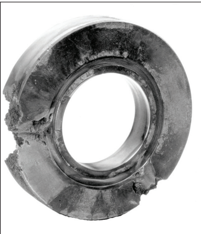
□ High pressure drop in globe valves can cause extreme cavitation damage such as shown on this globe valve seat. Proper material selection can help mitigate problems such as cavitation.
