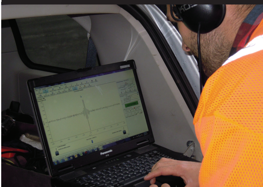
□ Acoustic leak detection offers a non-invasive detection method.
